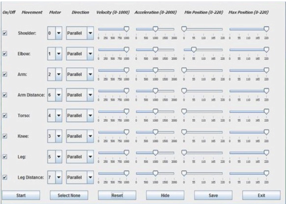
Figure 3 MOVE interface to mapping possibilities. The interface lets designers map body movements to prototype movements, allowing adjustments to panel velocity, acceleration, as well as min/max positions. Configuration can also be saved here.
